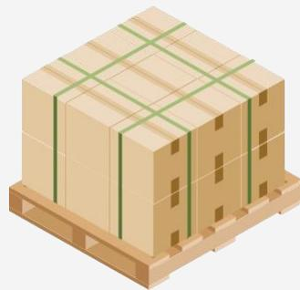
Use the retention straps (plastic or metal) properly to secure the load onto the base of the pallet. This provides the necessary structural sturdiness to ensure that your shipment will be handled and transported safely.
